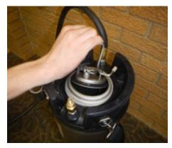
**3.** Push lid towards inside of tank and turn it sideways so it can easily be removed.
