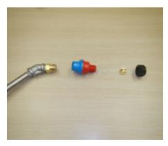
1. Attach black plastic cap with spray tip and clear plastic washer to the plastic CF Valve. Then attach CF Valve to brass 11/16" male fitting.
